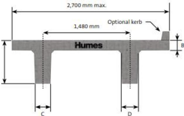
**Figure 3 – Cross-section detail of a complete HumeDeck® bridge system**
