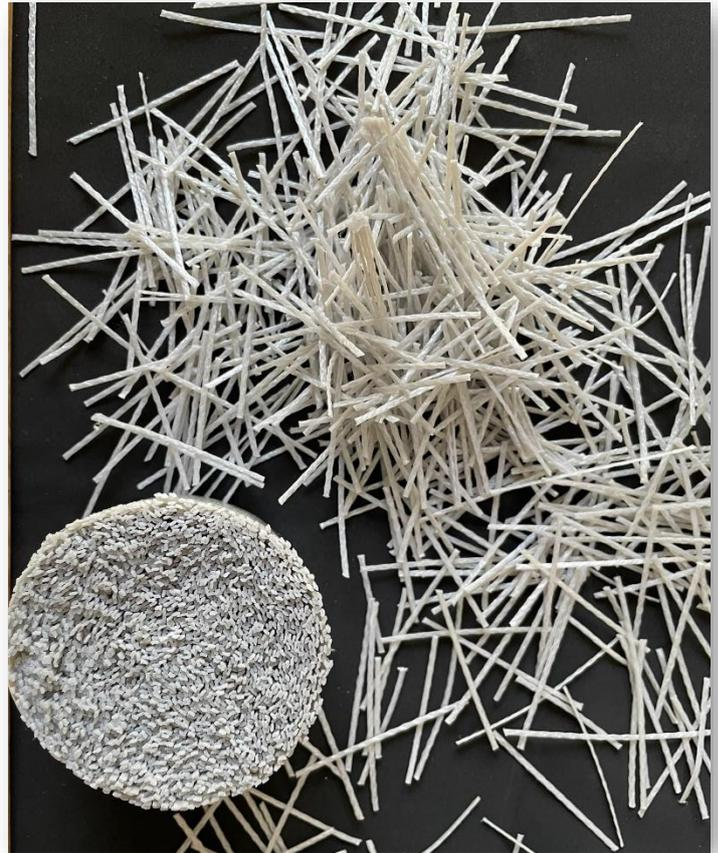
Virgin MSF are an ideal non-corrosive alternative to steel fibres with excellent post crack control (toughness) while being very economical and easy to use.
