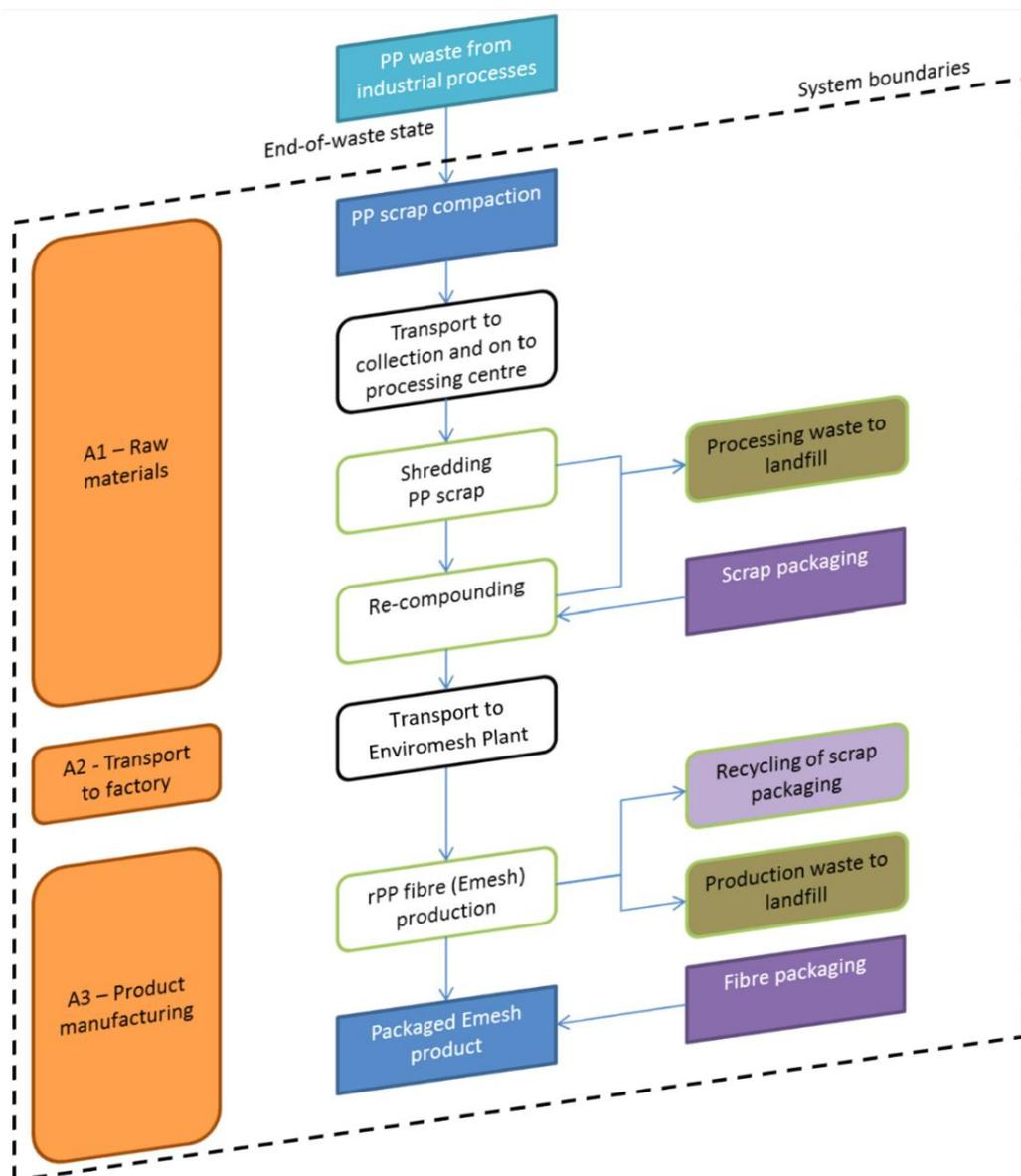
Figure 1. System boundaries for the eMesh LCA
