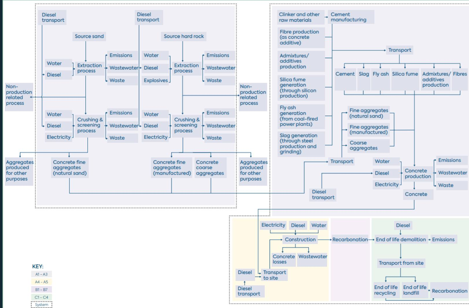
The lifecycle model and system boundary is the same for both Generic and Project-specific concrete EPDs, as detailed in the graphic.
