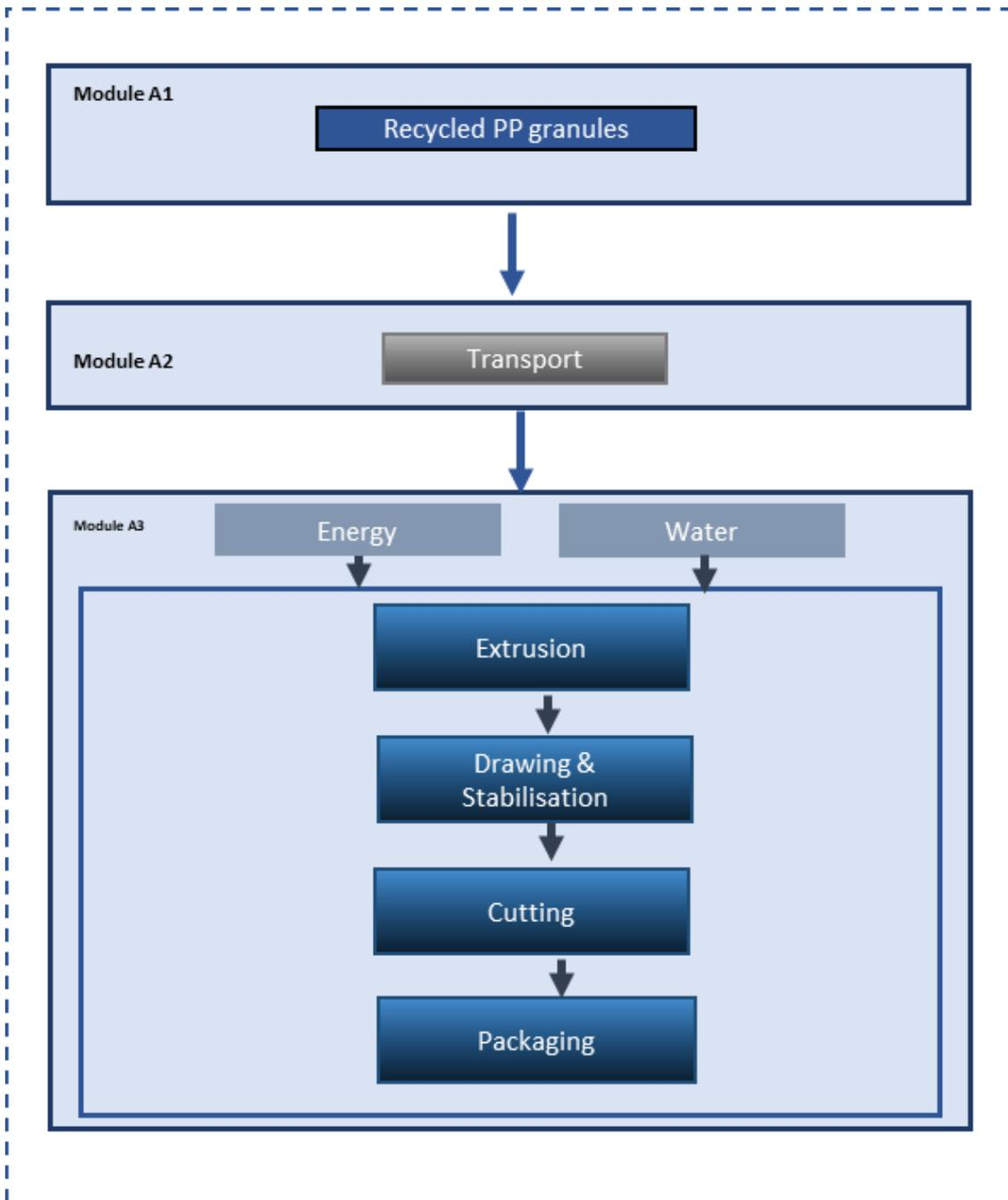
Figure 1 | Danbar Re-Poly RF47 EPD system boundary
