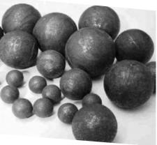
**Grinding media**Jused in the milling process
