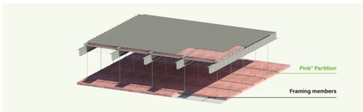
Diagram 2: Typical Ceiling Overlay Installation for Pink® Partition
