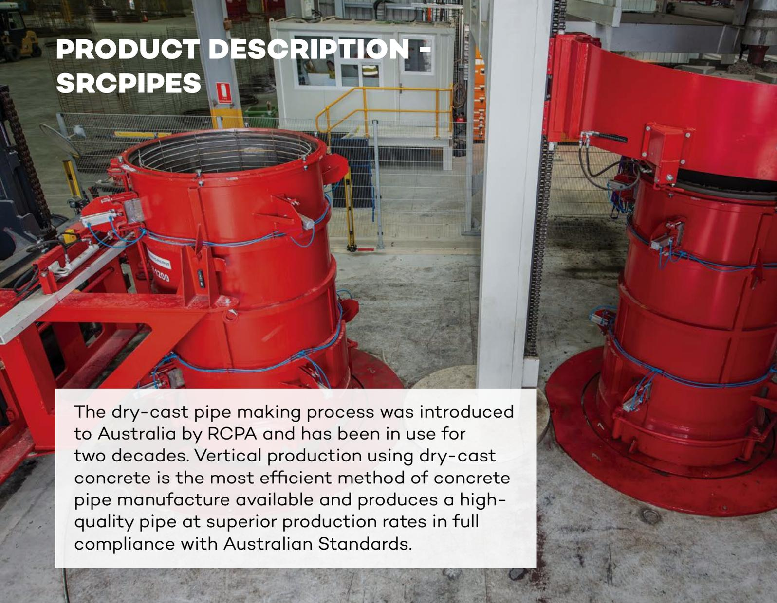
The dry-cast pipe making process was introduced to Australia by RCPA and has been in use for two decades. Vertical production using dry-cast concrete is the most efficient method of concrete pipe manufacture available and produces a high-quality pipe at superior production rates in full compliance with Australian Standards.
