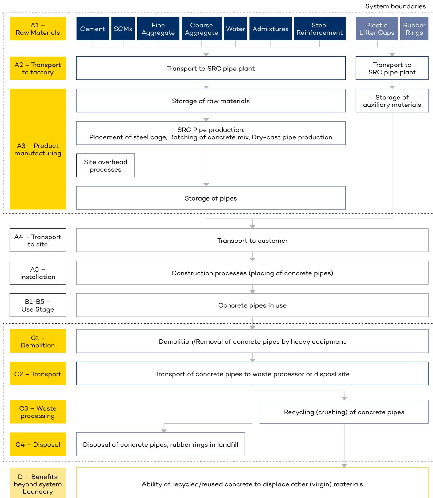
**Figure 3:** System boundary diagram of steel reinforced concrete pipes
